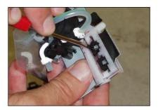
4. Now that the wiper blades are in place, connect the cap assembly to the pump assembly. Do this by connecting the black hose to the white coupler and then the white coupler to the clear hose with the green line coming out of the side of the pump assembly.
