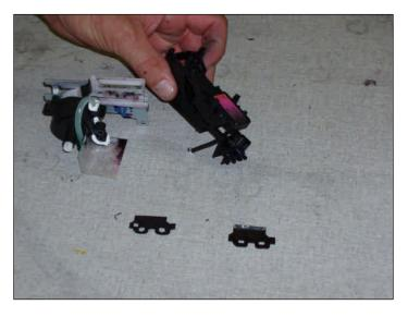
First install the wiper blades as shown in the picture on the right.
