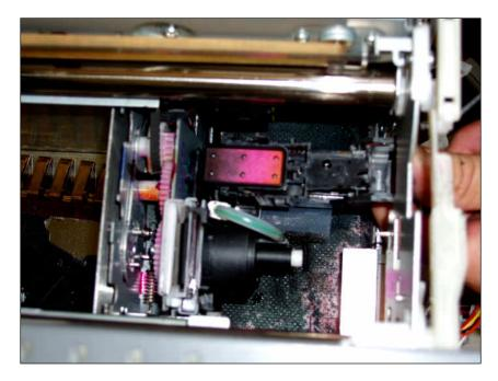
9. The final step is to put the screws back into the Capping/Pump assembly. Make sure that the Cap is assembly is on the out side of the machine when screwing it back in. As shown below.
