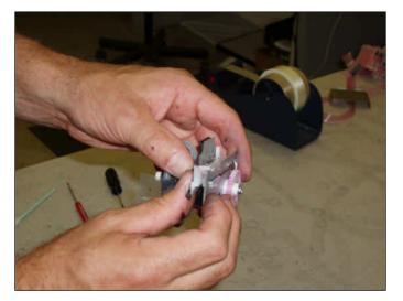
3. Use a small flat head screw driver to help mount the wiper blades onto the capping station. Make sure that the two openings at the bottom of the wiper blades fits securely over the two plastic grommets.
