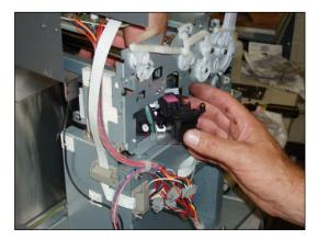
8. Position the capping/pump assembly carefully back into the machine and secure the silver plate with two screws. Check the top view to make sure everything is in place as shown below.
