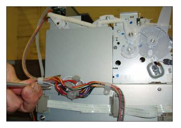
Remove the screws as identified on the right that are currently securing the capping station/pump assembly in place.
