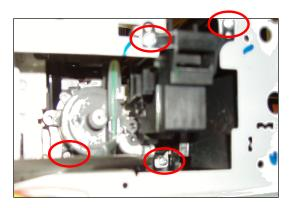
4. Both capping station/pump assembly can now be removed and to do so, there are two different methods in which you can follow – Removal from the top or removal from the side.
