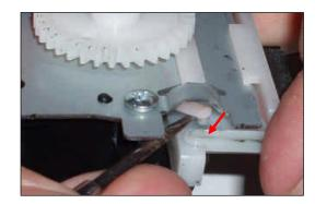
6. Once the wiper blade arm is in place, finish installing the cap assembly. There are two holes located on the silver plate that the capping assembly fits into. Move the wiper blade assembly all the way to the right for this step. When positioning the capping assembly in the silver plate, make sure that the white pin from the wiper blade assembly fits within the capping assembly as shown.
