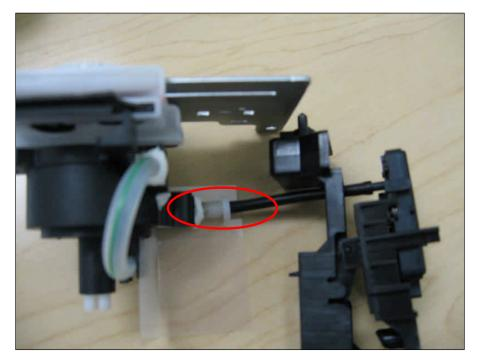
6. Make sure that the arm for the pumping station is properly attached to the wiper blade assembly. If the arm is not attached during a head cleaning, the pump assembly will make a grinding sound. Using a small flat head screw driver or pen, simply move the arm back into the grove on the wiper blade assembly.
