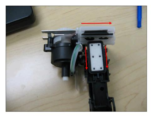
5. Remove the black line with the white coupler from the clear pump assembly ink tube.
