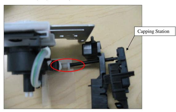
5. Make sure that the arm for the pumping station is properly attached to the wiper blade assembly. If the arm is not attached during a head cleaning, the pump assembly will make a grinding sound. Using a small flat head screw driver or pen, simply move the arm back into the grove on the wiper blade assembly.
