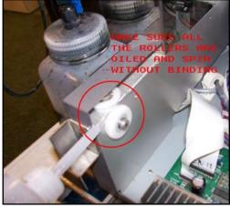
5. If you have a really dirty machine you may need to use a wire brush to clean the bar **under** the Yellow plate. To completely clean this bar, you must move the bed back and forth to get all of the dirt off the roller. Use care when cleaning this bar, there are electrical connections and printer components that can be damaged.
