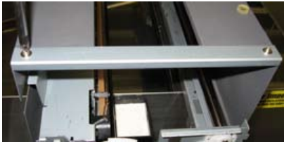
Step 3- Remove 2 screws from left cross brace
