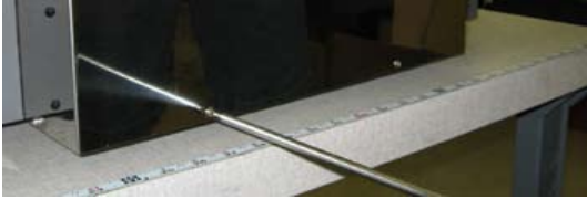
Step 1- Remove 4 screws from left side cover
