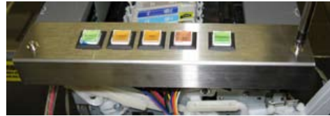
Step 4- Remove 2 screws from button bar
