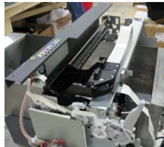
Printer with all necessary housing components removed
