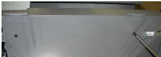
Step 5- Remove 2 screws from rear gray housing
