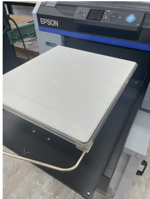
3. Adjust the platen height to the correct level. Once the film is correctly attached to the platen, check to make sure your platen height is on Level P (highest level to print).
