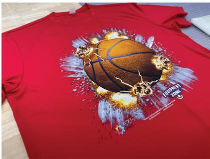
\* As the hot-melt DTF powder cools down, it acts as a binder that holds the colored pigment in the inks in firm adhesion with the fibers of the fabric.
