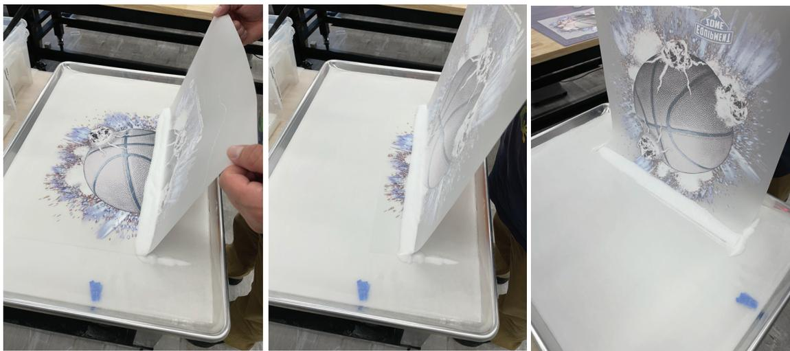
11. After dispersing the powder, give the film a good shake to remove all of the excess powder off of the film. If you do not shake it enough, after transferring you will see evidence of the powder around the image where there was not any ink printed.
