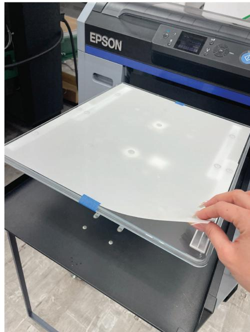
2. Center your film to the top of the platen. The end where the collar of a shirt would be.
