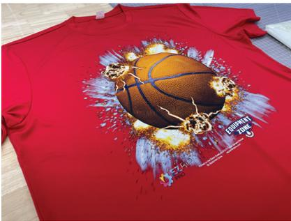
\* As the hot-melt DTF powder cools down, it acts as a binder that holds the colored pigment in the inks in firm adhesion with the fibers of the fabric.
