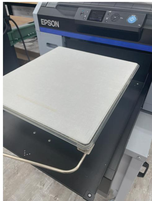
13. Adjust the platen height to the correct level. Once the film is correctly attached to the platen, check to make sure your platen height is on Level P (highest level to print).
