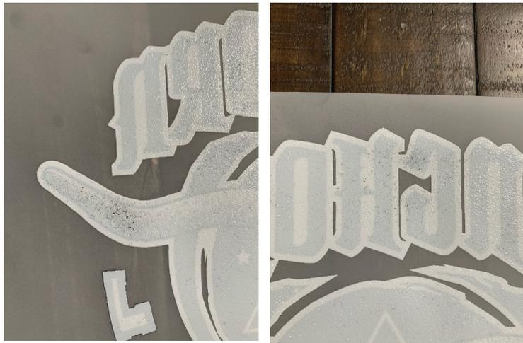
Be sure NOT to immediately put the powder onto the ink. This may cause the powder to seep through the ink and show after transferring. Color ink may appear to be faded out.
