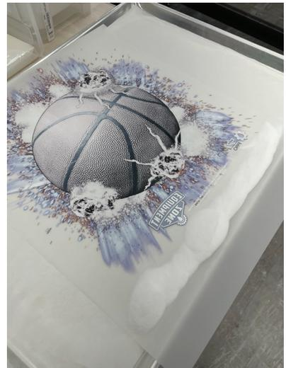
25. Carefully lift the film to disperse the powder all over the ink and off the film.
