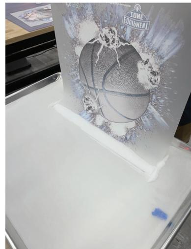
26. After dispersing the powder, give the film a good shake to remove all of the excess powder off of the film. If you do not shake it enough, after transferring you will see evidence of the powder around the image where there was not any ink printed.
